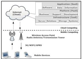
Fig. 3: Architecture of Mobile Cloud Computing
